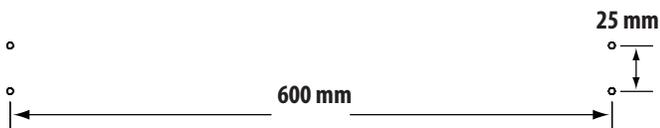
**NOTE:** To ensure the SB26 to be in level, use a carpenter's level, laser sight or another device to make the two sets of holes exactly at the same height.
